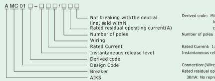
Derived code: Miniature Circuit Breaker: no representation; small leakage circuit breakers: The "E", said; small voltage
